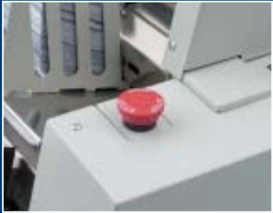
Emergency stop button for operator safety.
